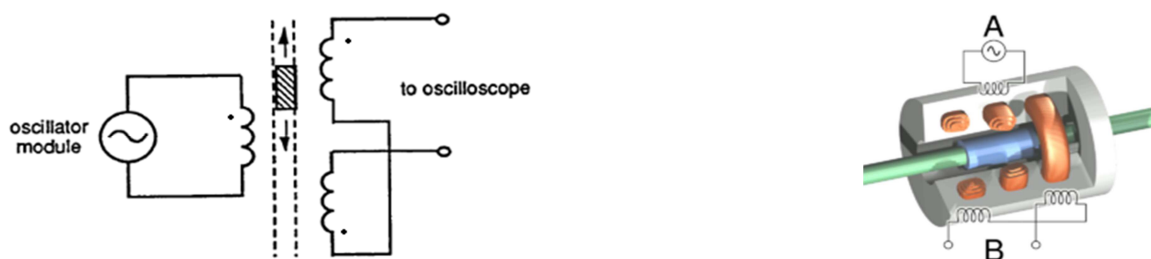
Figure: 1.1 LVDT setup and wiring
